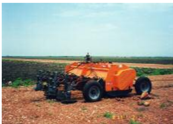
Removal of Cotton Stalks (Root Cutter)
